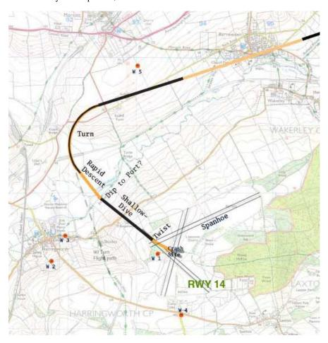
The A/c stalled out of a turn in line with a runway and had lost enough height so that, with a stall recovery (rapid descent) and a final adjustment of course, ended up in an 18 second slow, shallow descent, in line with a runway, with the engines idling, in other words what you do in a glide approach to a landing.
